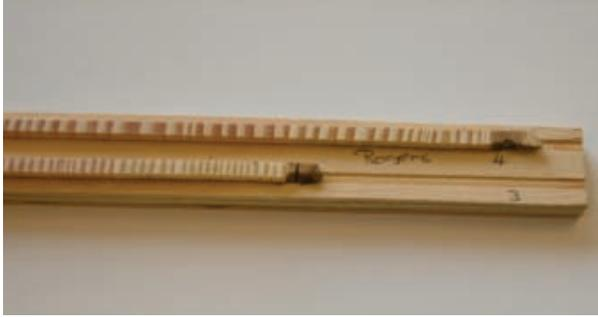
FIGURE 8 A wooden mount with two sanded cores.
