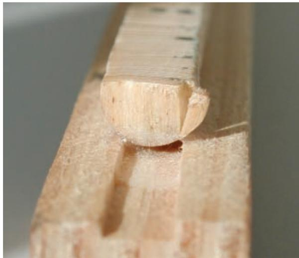
FIGURE 6 *An end-view of a sanded core showing vertical orientation of wood fibres.*
