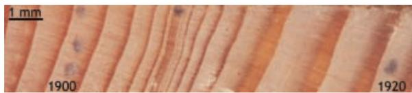
FIGURE 10 A close-up of an increment core from a spruce (*Picea glauca*), showing abrupt reduced growth and the system of noting years. Abrupt negative growth changes began in 1903 and continued until 1915. Growth was normal in 1916, then increased. These growth responses were due to deep burial by flood sediments, subsequent establishment of adventitious roots, and reduced competition (the event resulted in a 200 m wide swath cleared adjacent to the tree).
